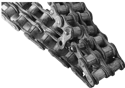
Corrosion of Stainless Steel Drive Chain
