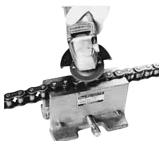
Figure 7: Grinding Down Pin Ends
