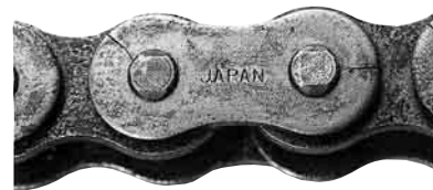
Hydrogen Embrittlement Cracking
