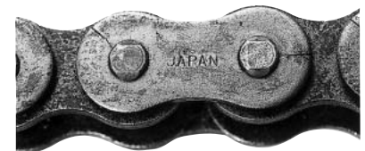
Fig. 32. Hydrogen embrittlement cracking
