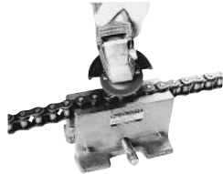
Fig. 2 Grinding the pin ends
