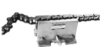
Fig. 3 Setting the roller chain in the chain vice
