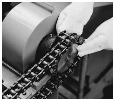
Fig. 8 Connecting on a sprocket
