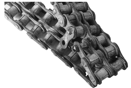
Fig. 31 Corrosion of stainless steel roller chain
