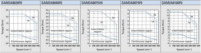
Note: GAM2A8075\* and GAM2A8100\* models may be derated with brake or oil seal.
