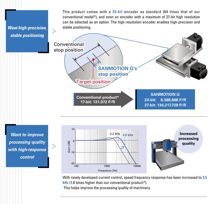
By accurately detecting and compensating for Coulomb friction, viscous friction, and the force of gravity, the positioning settling time has been made 1/3 that of our conventional product.\*
