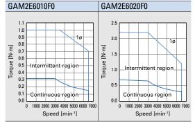
Note 1: Speed-torque characteristics curves and values in the row with a black star symbol (\*) are the values after thermal equilibrium is established. All other values are at a temperature of 20°C.
