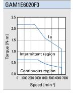
Note 1: Speed-torque characteristics curves and values in the row with a black star symbol (\*) are the values after thermal equilibrium is established. All other values are at a temperature of 20°C.
