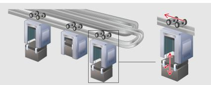
Servo systems are used to move conveyor trolleys, and grab and move up and down the boxes containing semiconductor wafers, making efficient semiconductor manufacturing possible.
