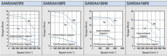
3ø: When the power supply voltage is 3-phase
