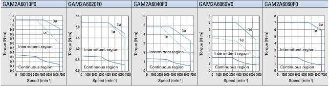
Note: GAM2A6040\* and GAM2A6060\* models may be derated with brake or oil seal.
