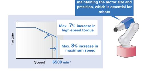
The servo motor's maximum speed has been increased from 6000 min<sup>-1</sup> to 6500 min<sup>-1</sup> compared to our conventional product.\* Also, the new PWM control has increased the maximum output torque at high speeds by approximately 7%, expanding the motor output range by up to 15%.
