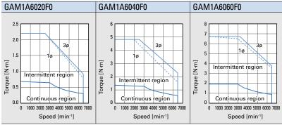
Note: GAM1A6040\* and GAM1A6060\* models may be derated with brake or oil seal. 3ø: When the power supply voltage is 3-phase
