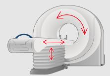
Servo systems are used for the gantry drive axis, and the vertical and horizontal bed moving axes. This application requires high vibration resistance and smooth motion.
