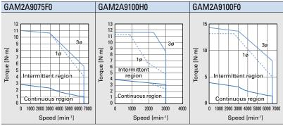
Note: GAM2A9100\* models may be derated with brake or oil seal.
