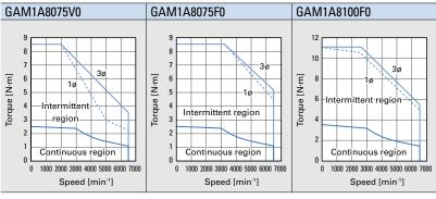
Note: GAM1A8075\* models may be derated with brake or oil seal.
