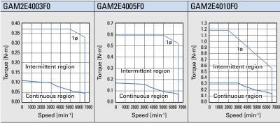
Note 1: Speed-torque characteristics curves and values in the row with a black star symbol (\*) are the values after thermal equilibrium is established. All other values are at a temperature of 20°C.
