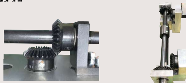
SM and SMB miters used to drive X/Y axes and transmit mechanical power
