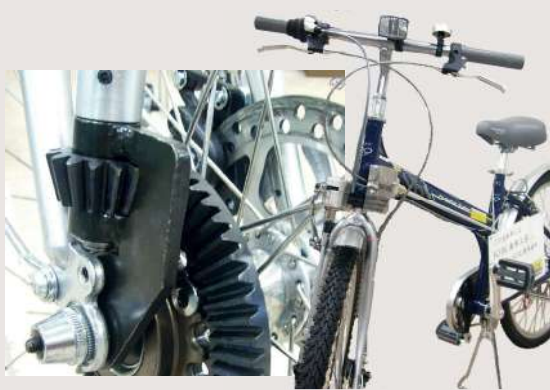
SB Bevel Gears are used in the driving components in both the front and rear wheels
