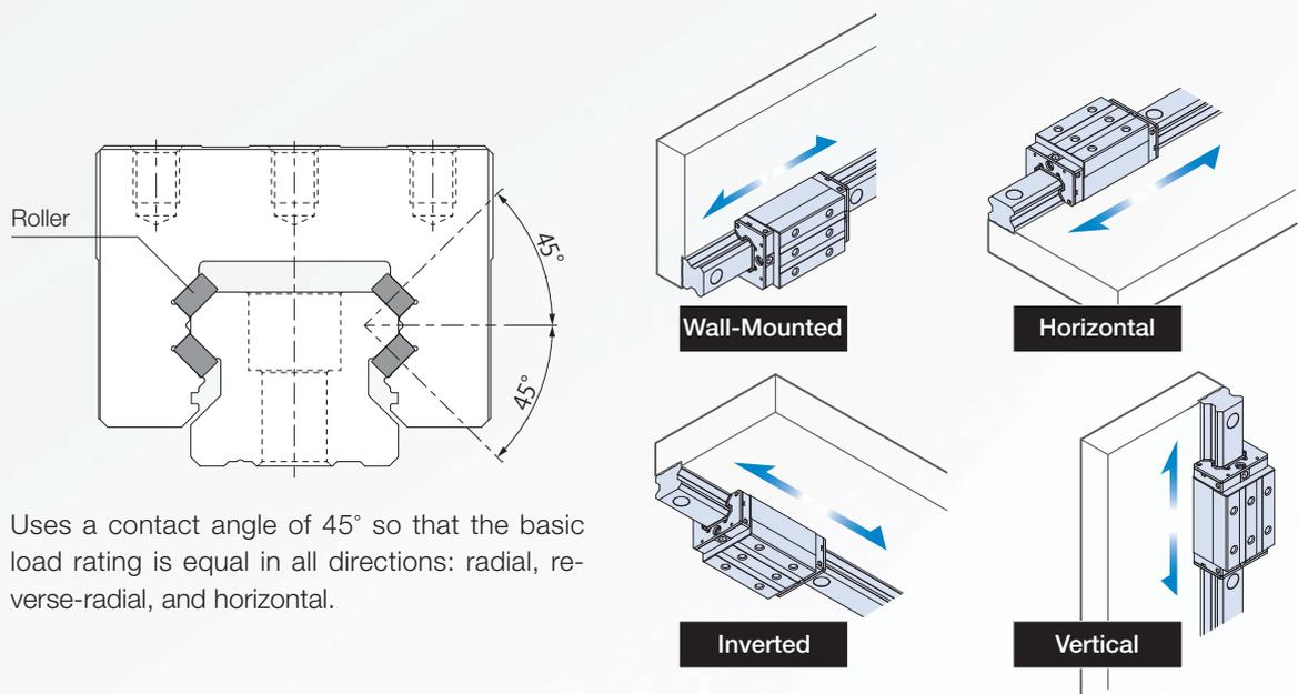
Uses a contact angle of 45° so that the basic load rating is equal in all directions: radial, reverse-radial, and horizontal.
