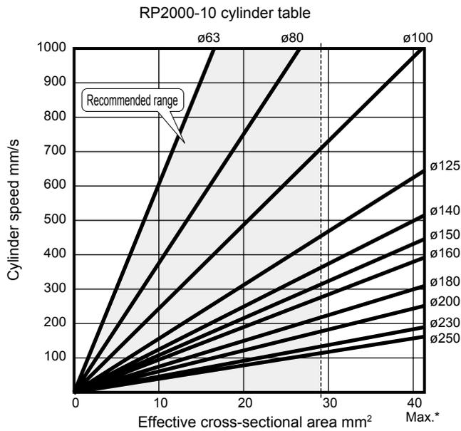
This cylinder table shows the available range according to the air supply and exhaust flow rate of the precision regulator and the required consumption flow rate at the cylinder PUSH/PULL.
