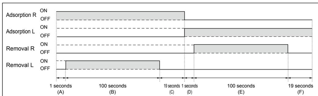
The normal processes are listed on the left. During energy conservation, the state (C, F) after the removal has been completed will be retained. After this, as soon as the dew point degrades, switching will resume to return to the normal processes.
