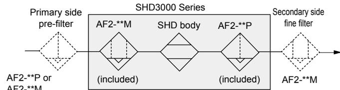
Assuming use with a line of a lubrication air compressor, although the SHD3000 Series is included with the AF2-\*\*M type for the primary side of the heatless dryer and the AF2-\*\*P type for the secondary side, as needed, separately install a primary side pre-filter or a secondary side fine filtration filter.
