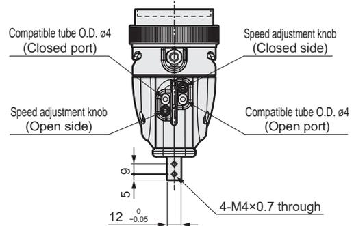
Dimensions when attachment is installed
