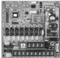
Sequential fluid control components for large port size dust collector valve
